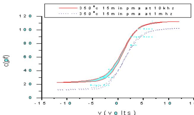
**Figure 7: C-V characteristics of InP MIS device**
