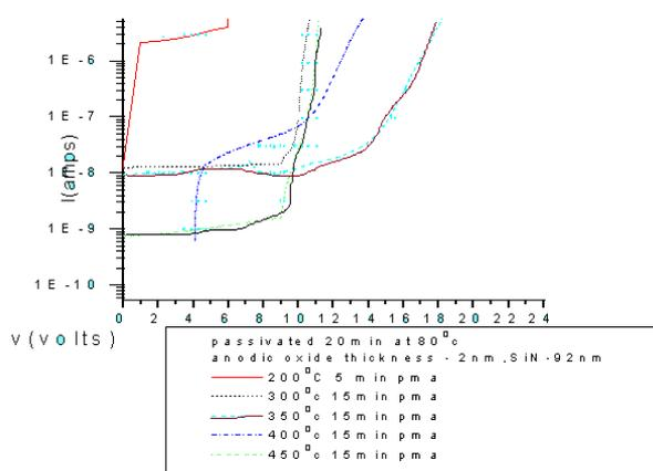
**Figure 6: I-V characteristics of InP MIS**
