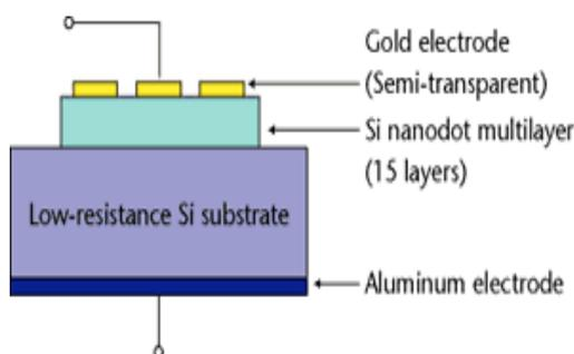
**Figure 4: Si Nano dot Fabrication.**
